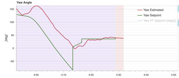
Figure 4: A Deviation-Type UAV Anomaly
